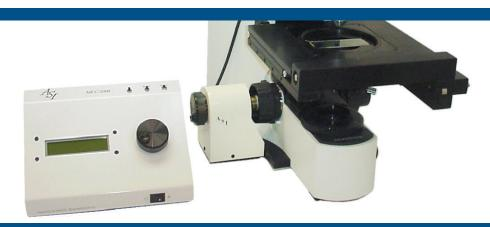
The MFC-2000 has been specifically designed to provide a high resolution and highly repeatable, means of controlling the focus/Z position of the microscope stage. Precise control of the microscope's focus is obtained through the use of a closed-loop DC servomotor employing high resolution encoders for positioning feedback. By using closed-loop control of the focus position, there is no chance that the focus point can be lost as can occur with open-loop stepper motors.
