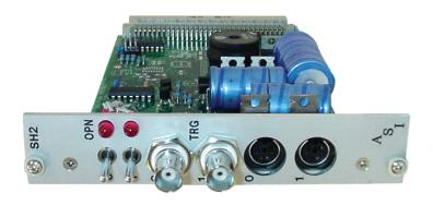
The SH-2 shutter card allows you to control the operation of two ASI shutters, and takes up a single slot in the PWR-ASI-6 power supply. Typically the SH-2 is used along with other modules, such as the FW-1000 filter wheel controller.
