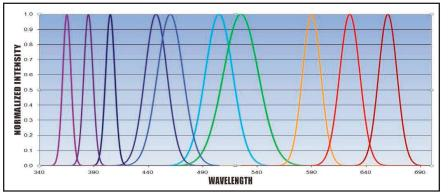
Eleven different LEDs are available. The 10 LEDs above each provide a narrow spectrum of light for specific fluorescent purposes. A white light LED is also available, giving a broad spectrum of light.
