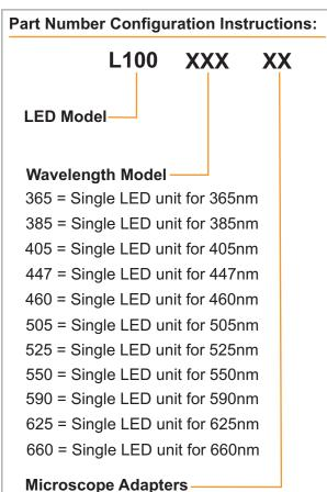
LC = Adapter for Leica microscopes NI = Adapter for Nikon microscopes OL = Adapter for Olympus microscopes ZS = Adapter for Zeiss microscopes
